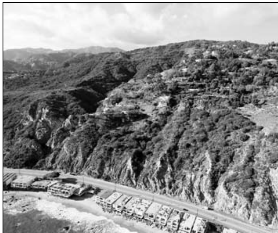
Slope ordinances got their start in the Los Angeles area, where development along steep canyon rims often led to landslides in wet weather.
