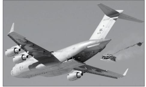
The C-17, shown above, is a strategic jet transport capable of hauling larger payloads, such as a tank or a larger number of troops, over greater distances than the turboprop-powered C-130. (Pixabay photo)
